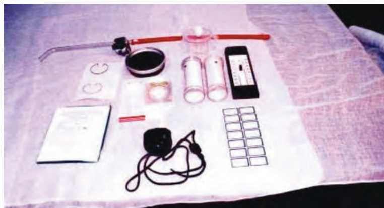
Figure An4.1 Equipment for susceptibility testing with a box of insecticide impregnated paper
