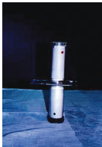
Figure An4.5 Exposure tubes held at vertical position
